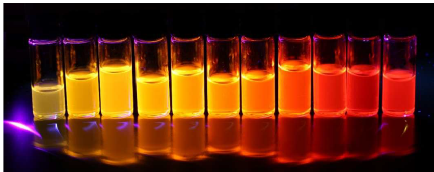
Figure 1. Size-separated silicon nanocrystals dispersed in toluene showing intense luminescence from the deep red to the yellow spectral region. Excitation: (a) 365 nm LED.
