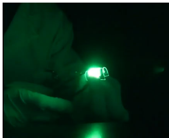
Figure 4. Photograph of device performance of LED fabricated on PET in operation.
